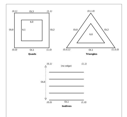
Figure 2.7. Domain parameterization for tessellation generator primitive modes (triangles, quads, or isolines). The coordinates illustrate the value of  ${\tt gl\_TessCoord}$  at the corners of the domain. The labels on the edges indicate the inner (ILO and IL1) and outer (OL0 through OL3) tessellation level values used to control the number of subdivisions along each edge of the domain.
