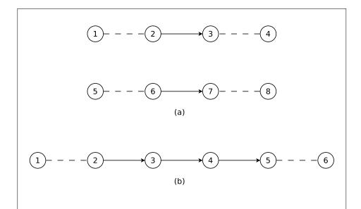
Figure 2.4. Lines with adjacency (a) and line strips with adjacency (b). The vertices connected with solid lines belong to the main primitives; the vertices connected by dashed lines are the adjacent vertices that may be used in a geometry shader.
