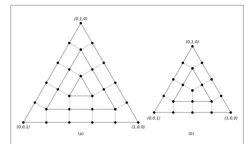
Figure 2.8. Inner triangle tessellation with inner tessellation levels of (a) five and (b) four, respectively (not to scale) Solid black circles depict vertices along the bottom edges of the concentric triangles. The edges of inner triangles are subdivided by intersecting the edge with segments perpendicular to the edge passing through each inner vertex of the subdivided outer edge. Dotted lines depict edges connecting corresponding vertices on the inner and outer triangle edges.
