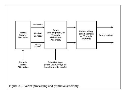
coordinates and varying vertex shader outputs. In the case of line and polygon primitives, clipping may insert new vertices into the primitive. The vertices defining a primitive to be rasterized have varying outputs associated with them.
