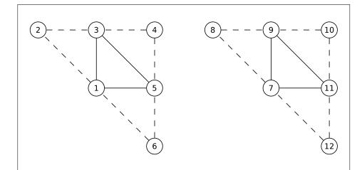
Figure 2.5. Triangles with adjacency. The vertices connected with solid lines belong to the main primitive; the vertices connected by dashed lines are the adjacent vertices that may be used in a geometry shader.
