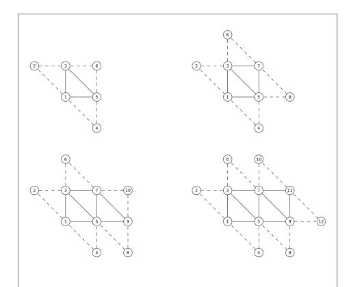
Figure 10.8. Triangle strips with adjacency. The vertices connected with solid lines belong to the main primitives; the vertices connected by dashed lines are the adjacent vertices that may be used in a geometry shader.
