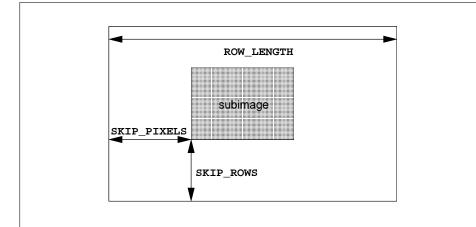
Figure 8.2. Selecting a subimage from an image. The indicated parameter names are prefixed by UNPACK\_ for **DrawPixels** and by PACK\_ for **ReadPixels**.
