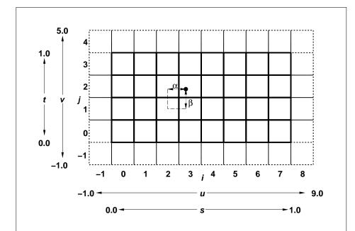
Figure 8.3. A texture image and the coordinates used to access it. This is a two-dimensional texture with *width* 8 and *height* 4. A one-dimensional texture would consist of a single horizontal strip.  $\alpha$  and  $\beta$ , values used in blending adjacent texels to obtain a texture value are also shown.
