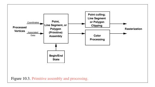
vertex processing. The vertices defining a primitive to be rasterized have vertex coordinates, texture coordinates and colors associated with them. After a primitive is formed, clipping may alter all these attributes.
