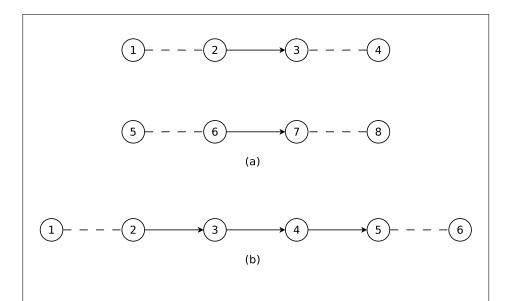
Figure 10.6. Lines with adjacency (a) and line strips with adjacency (b). The vertices connected with solid lines belong to the main primitives; the vertices connected by dashed lines are the adjacent vertices that may be used in a geometry shader.
