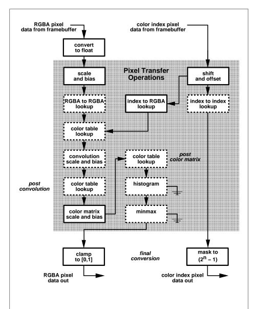
Figure 18.2. Operation of **CopyPixels**. Operations in dashed boxes may be enabled or disabled. Index-to-RGBA lookup is currently never performed. RGBA and color index pixel paths are shown; depth and stencil pixel paths are not shown.
