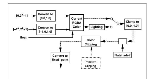
Figure 12.2. Processing of RGBA colors. The heavy dotted lines indicate both primary and secondary vertex colors, which are processed in the same fashion. k is the minimum required bit width of the integer type representing a color component.
