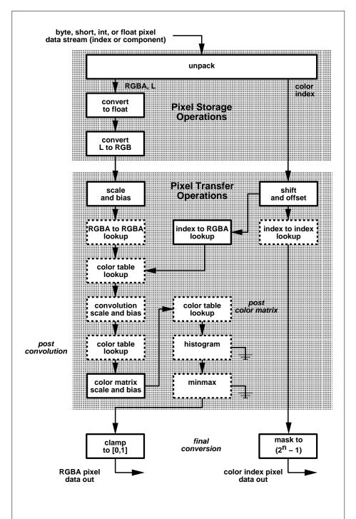
Figure 8.1. Transfer of pixel rectangles to the GL. Output is RGBA pixels if the GL is in RGBA mode, color index pixels otherwise. Operations in dashed boxes may be enabled OpenGLe4.4R(Compatibility Profile)xelMatchat9,s2044; depth and stencil pixel paths are not shown.
