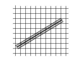
Figure 14.6. The region used in rasterizing and finding corresponding coverage values for an antialiased line segment (an x-major line segment is shown).
