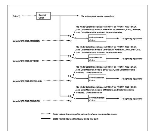
Figure 12.4. ColorMaterial operation. Material properties are continuously updated from the current color while ColorMaterial is enabled and has the appropriate mode. Only the front material properties are included in this figure. The back material properties are treated identically, except that *face* must be BACK or FRONT\_AND\_BACK.
