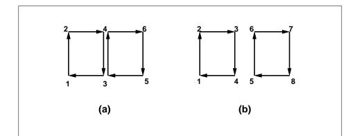
Figure 10.5. (a) A quad strip. (b) Independent quads. The numbers give the sequencing of the vertices passed to the GL.
