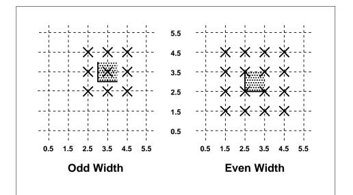
**Figure 14.2.** Rasterization of non-antialiased wide points. The crosses show fragment centers produced by rasterization for any point that lies within the shaded region. The dotted grid lines lie on half-integer coordinates.
