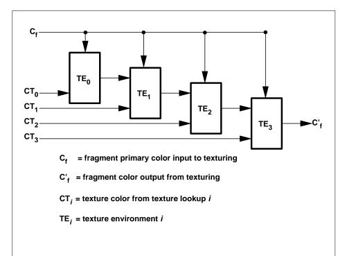
Figure 16.1. Multitexture pipeline. Four texture units are shown; however, multitexturing may support a different number of units depending on the implementation. The input fragment color is successively combined with each texture according to the state of the corresponding texture environment, and the resulting fragment color passed as input to the next texture unit in the pipeline.
