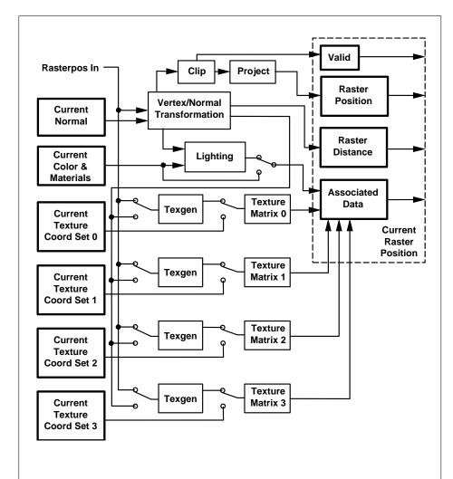
Figure 14.7. The current raster position and how it is set. Four texture units are shown; however, multitexturing may support a different number of units depending on the implementation.
