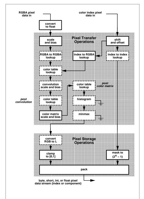
Figure 18.1. Operation of **ReadPixels**. Operations in dashed boxes may be enabled or disabled, except in the case of "convert RGB to L", which is only applied when reading color data in luminosity formats. RGBA and color index pixel paths are shown; depth and stencil pixel paths are not shown.
