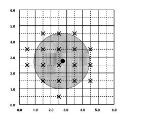
**Figure 14.3.** Rasterization of antialiased wide points. The black dot indicates the point to be rasterized. The shaded region has the specified width. The X marks indicate those fragment centers produced by rasterization. A fragment's computed coverage value is based on the portion of the shaded region that covers the corresponding fragment square. Solid lines lie on integer coordinates.
