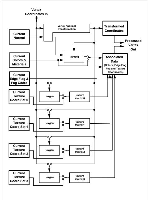
Figure 10.2. Association of current values with a vertex. The heavy lined boxes represent GL state. Four texture units are shown; however, multitexturing may support a different number of units depending on the implementation.
