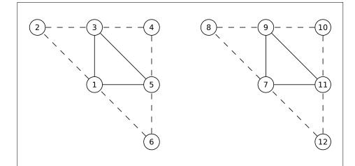
Figure 10.7. Triangles with adjacency. The vertices connected with solid lines belong to the main primitive; the vertices connected by dashed lines are the adjacent vertices that may be used in a geometry shader.
