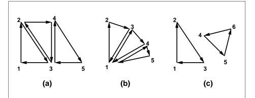
Figure 2.4. (a) A triangle strip. (b) A triangle fan. (c) Independent triangles. The numbers give the sequencing of the vertices in order within the vertex arrays. Note that in (a) and (b) triangle edge ordering is determined by the first triangle, while in (c) the order of each triangle's edges is independent of the other triangles.
