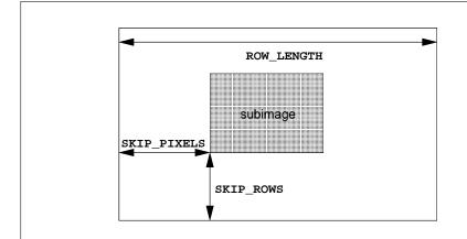
Figure 3.5. Selecting a subimage from an image. The indicated parameter names are prefixed by UNPACK\_ for **TexImage\*** and by PACK\_ for **ReadPixels**.
