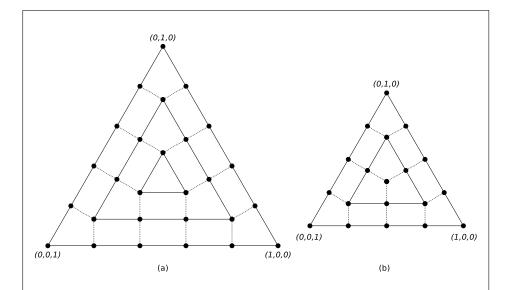
Figure 2.8. Inner triangle tessellation with inner tessellation levels of (a) five and (b) four, respectively (not to scale) Solid black circles depict vertices along the edges of the concentric triangles. The edges of inner triangles are subdivided by intersecting the edge with segments perpendicular to the edge passing through each inner vertex of the subdivided outer edge. Dotted lines depict edges connecting corresponding vertices on the inner and outer triangle edges.
