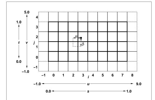
Figure 3.6. A texture image and the coordinates used to access it. This is a two-dimensional texture with n=3 and m=2. A one-dimensional texture would consist of a single horizontal strip.  $\alpha$  and  $\beta$ , values used in blending adjacent texels to obtain a texture value, are also shown.
