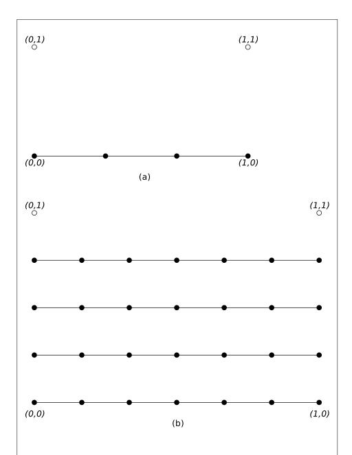
Figure 2.10. Isoline tessellation with the first two outer tessellation levels of (a) (3,1) and (b) (6,4), respectively. Line segments connecting the vertices marked with solid black circles are emitted by the primitive generator. Vertices marked with empty circles correspond to (u,v) coordinates of (0,1) and (1,1), where no line segments are generated.
