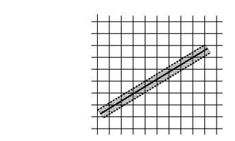
Figure 3.3. The region used in rasterizing and finding corresponding coverage values for an antialiased line segment (an x-major line segment is shown).
