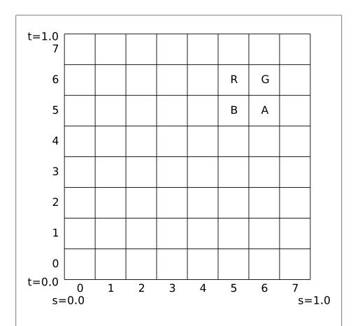
Figure 3.7. An example of an  $8\times 8$  texture image and the components returned for textureGather.
