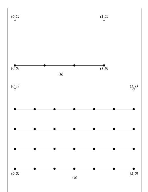
Figure 2.16. Isoline tessellation with the first two outer tessellation levels of (a) (3,1) and (b) (6,4), respectively. Line segments connecting the vertices marked with solid black circles are emitted by the primitive generator. Vertices marked with empty circles correspond to (u,v) coordinates of (0,1) and (1,1), where no line segments are generated.
