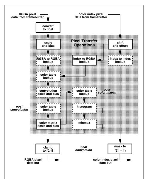
Figure 4.3. Operation of **CopyPixels**. Operations in dashed boxes may be enabled or disabled. Index-to-RGBA lookup is currently never performed. RGBA and color index pixel paths are shown; depth and stencil pixel paths are not shown.
