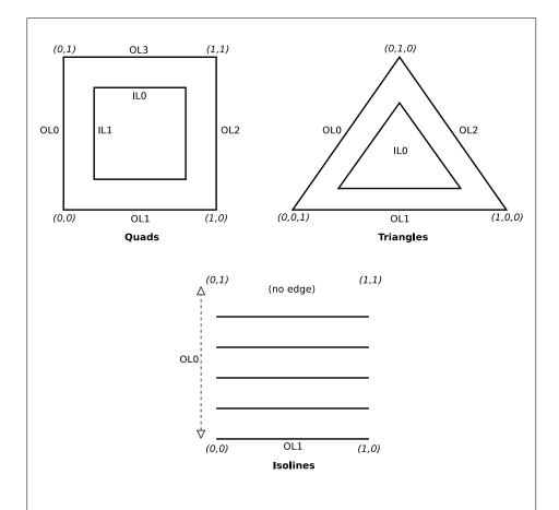
Figure 2.13. Domain parameterization for tessellation generator primitive modes (triangles, quads, or isolines). The coordinates illustrate the value of gl\_- TessCoord at the corners of the domain. The labels on the edges indicate the inner (IL0 and IL1) and outer (OL0 through OL3) tessellation level values used to control the number of subdivisions along each edge of the domain.
