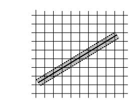
Figure 3.6. The region used in rasterizing and finding corresponding coverage values for an antialiased line segment (an x-major line segment is shown).
