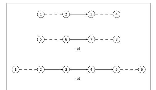
Figure 2.6. Lines with adjacency (a) and line strips with adjacency (b). The vertices connected with solid lines belong to the main primitives; the vertices connected by dashed lines are the adjacent vertices that may be used in a geometry shader.
