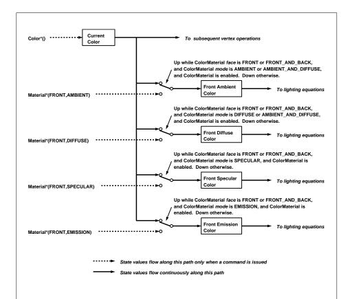
Figure 2.12. ColorMaterial operation. Material properties are continuously updated from the current color while ColorMaterial is enabled and has the appropriate mode. Only the front material properties are included in this figure. The back material properties are treated identically, except that *face* must be BACK or FRONT\_AND\_BACK.
