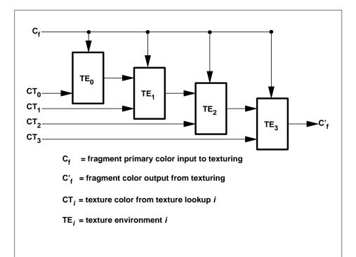
Figure 3.12. Multitexture pipeline. Four texture units are shown; however, multitexturing may support a different number of units depending on the implementation. The input fragment color is successively combined with each texture according to the state of the corresponding texture environment, and the resulting fragment color passed as input to the next texture unit in the pipeline.
