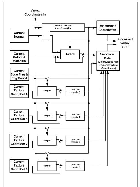
Figure 2.2. Association of current values with a vertex. The heavy lined boxes represent GL state. Four texture units are shown; however, multitexturing may support a different number of units depending on the implementation.
