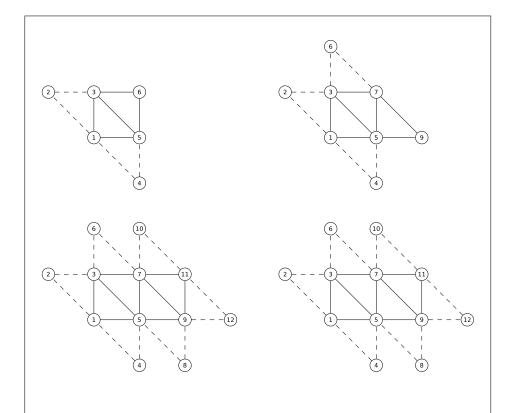
Figure 2.8. Triangle strips with adjacency. The vertices connected with solid lines belong to the main primitives; the vertices connected by dashed lines are the adjacent vertices that may be used in a geometry shader.
