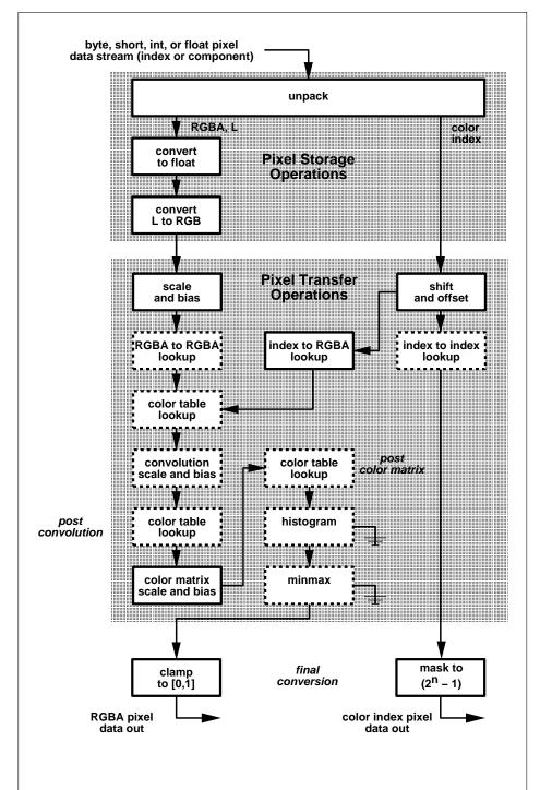
Figure 3.7. Transfer of pixel rectangles to the GL. Output is RGBA pixels if the GL is in RGBA mode, color index pixels otherwise. Operations in dashed boxes may be enabled or OpenGB 4.10 (Compatibility Profile) of July 25; 2010 n; depth and stencil pixel paths are not shown.
