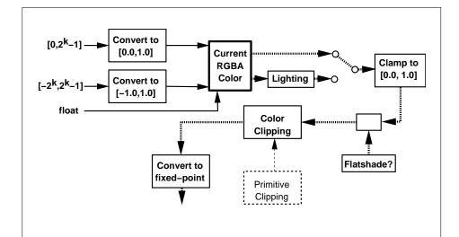
Figure 2.10. Processing of RGBA colors. The heavy dotted lines indicate both primary and secondary vertex colors, which are processed in the same fashion. k is the minimum required bit width of the integer type representing a color component.
