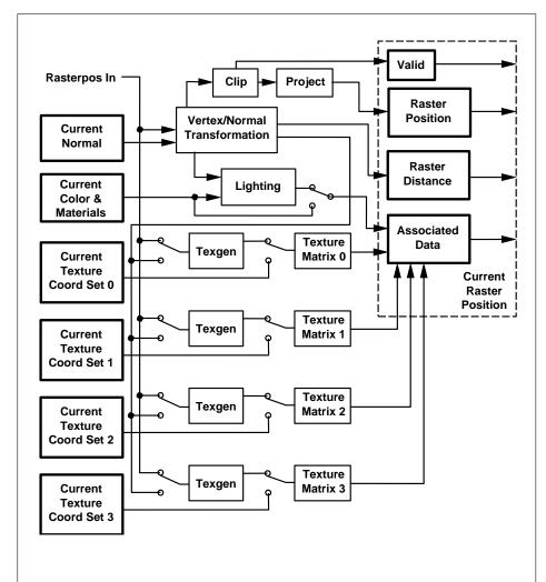
Figure 2.17. The current raster position and how it is set. Four texture units are shown; however, multitexturing may support a different number of units depending on the implementation.
