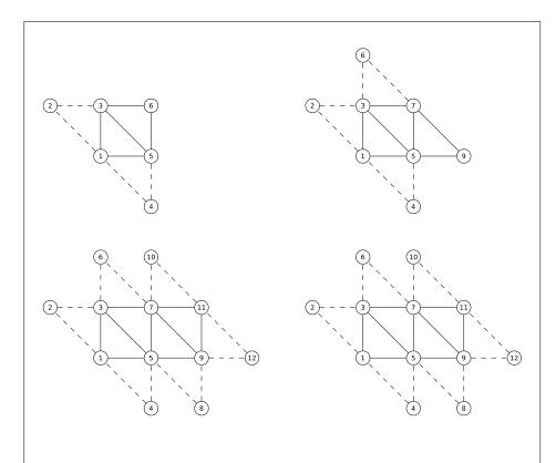
Figure 2.6. Triangle strips with adjacency. The vertices connected with solid lines belong to the main primitives; the vertices connected by dashed lines are the adjacent vertices that may be used in a geometry shader.
