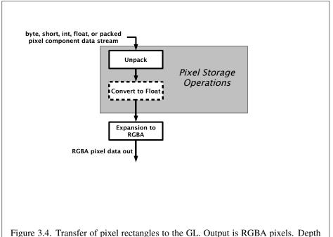
Figure 3.4. Transfer of pixel rectangles to the GL. Output is RGBA pixels. Depth and stencil pixel paths are not shown.
