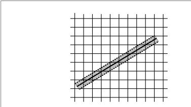
Figure 3.3. The region used in rasterizing and finding corresponding coverage values for an antialiased line segment (an x-major line segment is shown).
