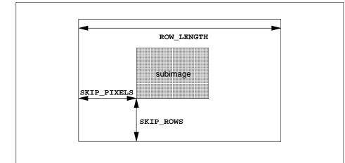
Figure 3.5. Selecting a subimage from an image. The indicated parameter names are prefixed by UNPACK\_ for **TexImage\*** and by PACK\_ for **ReadPixels**.
