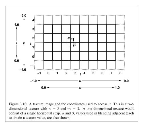
texture, j and k are both irrelevant). The *texture value* used in texturing a fragment is determined by that fragment's associated (s, t, r) coordinates in fixed-function fragment shading, or by sampling the texture in a shader, but may not correspond to any actual texel. See figure 3.10.
