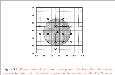
point to be rasterization of antialiased wide points. The black dot indicates the point to be rasterized. The shaded region has the specified width. The X marks indicate those fragment centers produced by rasterization. A fragment's computed coverage value is based on the portion of the shaded region that covers the corresponding fragment square. Solid lines lie on integer coordinates.
