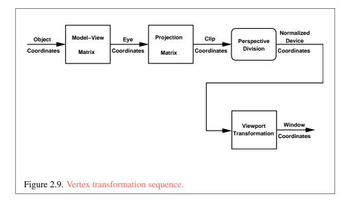
Object coordinates, eye coordinates, and clip coordinates are four-dimensional, consisting of x, y, z, and w coordinates (in that order). The model-view and projection matrices are thus  $4 \times 4$ .
