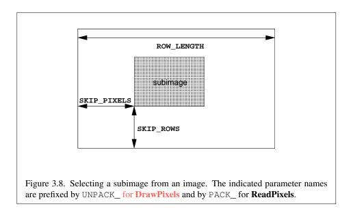
UNPACK\_ROW\_LENGTH, UNPACK\_SKIP\_ROWS, and UNPACK\_SKIP\_PIXELS. Before obtaining the first group from memory, the *data* pointer is advanced by  $(UNPACK_SKIP_PIXELS)n + (UNPACK_SKIP_ROWS)k$  elements. Then *width* groups are obtained from contiguous elements in memory (without advancing the pointer), after which the pointer is advanced by k elements. *height* sets of *width* groups of values are obtained this way. See figure 3.8.
