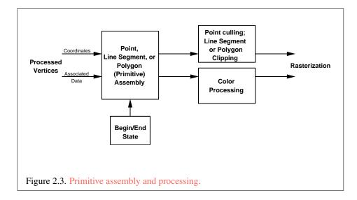
processing indicated for each current value is applied for each vertex that is sent to the GL.
