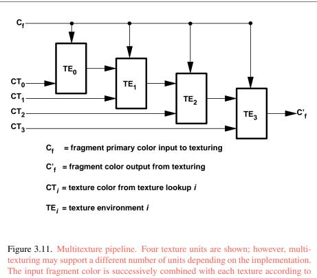
the state of the corresponding texture environment, and the resulting fragment color passed as input to the next texture unit in the pipeline.
