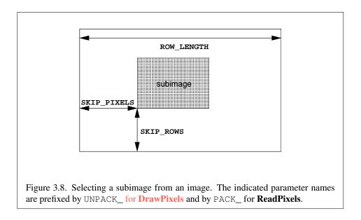
pointer), after which the pointer is advanced by k elements. *height* sets of *width* groups of values are obtained this way. See figure 3.8.
