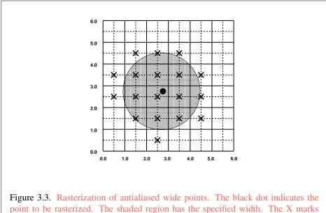
Figure 3.3. Rasterization of antialiased wide points. The black dot indicates the point to be rasterized. The shaded region has the specified width. The X marks indicate those fragment centers produced by rasterization. A fragment's computed coverage value is based on the portion of the shaded region that covers the corresponding fragment square. Solid lines lie on integer coordinates.
