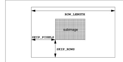
Figure 3.5. Selecting a subimage from an image. The indicated parameter names are prefixed by UNPACK\_ for **TexImage\*** and by PACK\_ for **ReadPixels**.
