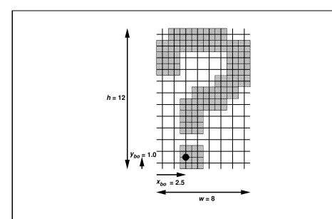
Figure 3.9. A bitmap and its associated parameters.  $x_{bi}$  and  $y_{bi}$  are not shown.
