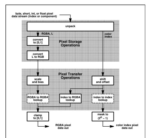
Figure 3.7. Operation of **DrawPixels**. Output is RGBA pixels if the GL is in RGBA mode, color index pixels otherwise. (Depth and stencil pixel paths are not illustrated.) RGBA-to-RGBA and index-to-index lookup are optional.
