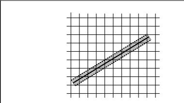
Figure 3.6. The region used in rasterizing and finding corresponding coverage values for an antialiased line segment (an x-major line segment is shown).
