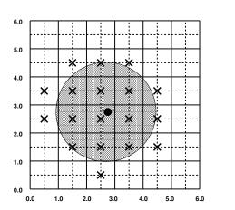
Figure 3.3. Rasterization of antialiased wide points. The black dot indicates the point to be rasterized. The shaded region has the specified width. The X marks indicate those fragment centers produced by rasterization. A fragment's computed coverage value is based on the portion of the shaded region that covers the corresponding fragment square. Solid lines lie on integer coordinates.
