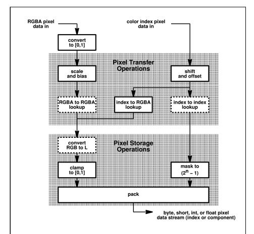
Figure 4.2. Operation of **ReadPixels**. RGBA and color index pixel paths are shown; depth and stencil pixel paths are not shown. RGBA-to-RGBA lookup, index-to-index lookup, and RGB-to-L conversion are optional.
