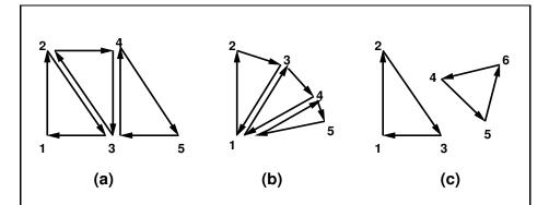
Figure 2.4. (a) A triangle strip. (b) A triangle fan. (c) Independent triangles. The numbers give the sequencing of the vertices between **Begin** and **End**. Note that in (a) and (b) triangle edge ordering is determined by the first triangle, while in (c) the order of each triangle's edges is independent of the other triangles.
