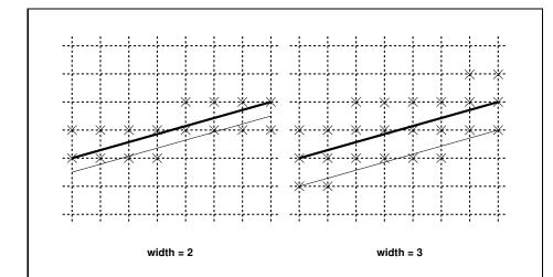
Figure 3.5. Rasterization of non-antialiased wide lines. x-major line segments are shown. The heavy line segment is the one specified to be rasterized; the light segment is the offset segment used for rasterization. x marks indicate the fragment centers produced by rasterization.
