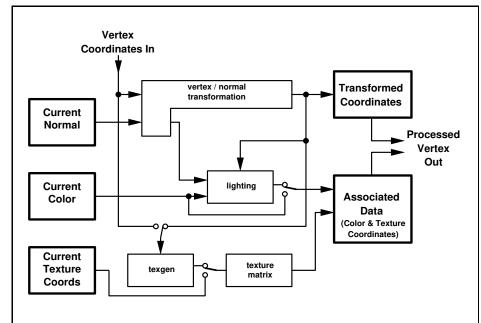
Figure 2.2. Association of current values with a vertex. The heavy lined boxes represent  $\operatorname{GL}$  state.
