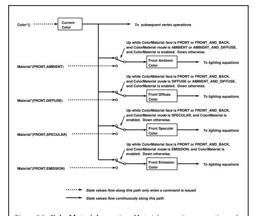
Figure 2.9. ColorMaterial operation. Material properties are continuously updated from the current color while ColorMaterial is enabled and has the appropriate mode. Only the front material properties are included in this figure. The back material properties are treated identically.
