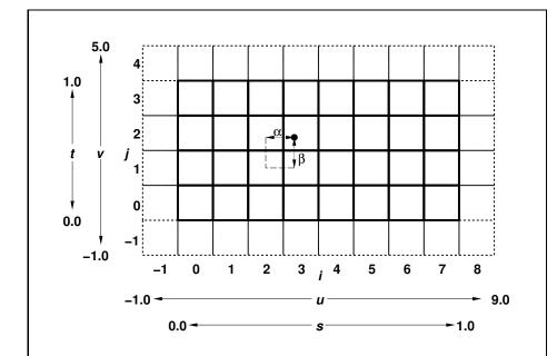
Figure 3.10. A texture image and the coordinates used to access it. This is a two-dimensional texture with n=3 and m=2. A one-dimensional texture would consist of a single horizontal strip.  $\alpha$  and  $\beta$ , values used in blending adjacent texels to obtain a texture value, are also shown.
