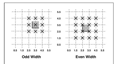
Figure 3.2. Rasterization of non-antialiased wide points. The crosses show fragment centers produced by rasterization for any point that lies within the shaded region. The dotted grid lines lie on half-integer coordinates.
