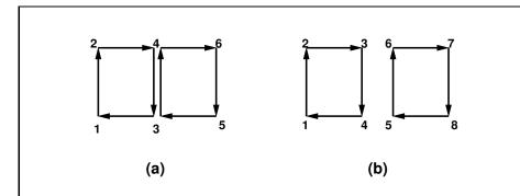
Figure 2.5. (a) A quad strip. (b) Independent quads. The numbers give the sequencing of the vertices between **Begin** and **End**.
