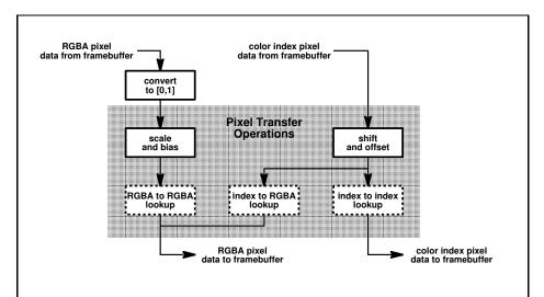
Figure 4.3. Operation of **CopyPixels**. RGBA and color index pixel paths are shown; depth and stencil pixel paths are not shown. RGBA-to-RGBA and index-to-index lookup are optional. Index-to-RGBA lookup is currently never performed.
