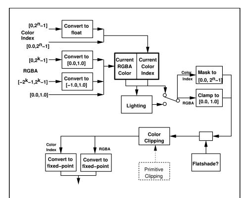
Figure 2.8. Processing of colors. n is the number of bits in a color index; m is the number of bits an R, G, B, or A component. See Table 2.6 for the interpretation of k.
