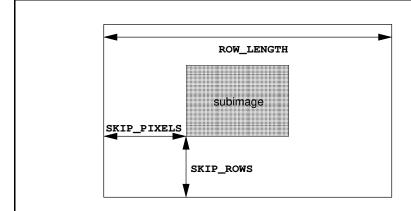
Figure 3.8. Selecting a subimage from an image. The indicated parameter names are prefixed by UNPACK\_ for **DrawPixels** and by PACK\_ for **ReadPixels**.
